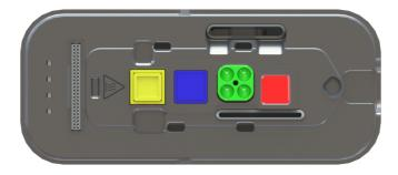
• The heater and peltier: (yellow and blue) - These heat the reagents for reactions and incubation stages of the library preparation. The peltier and heater will warm the reagents, while the former can cool the solution temperature too. These enable dual incubations and/or rapid changes between thermal environments.
